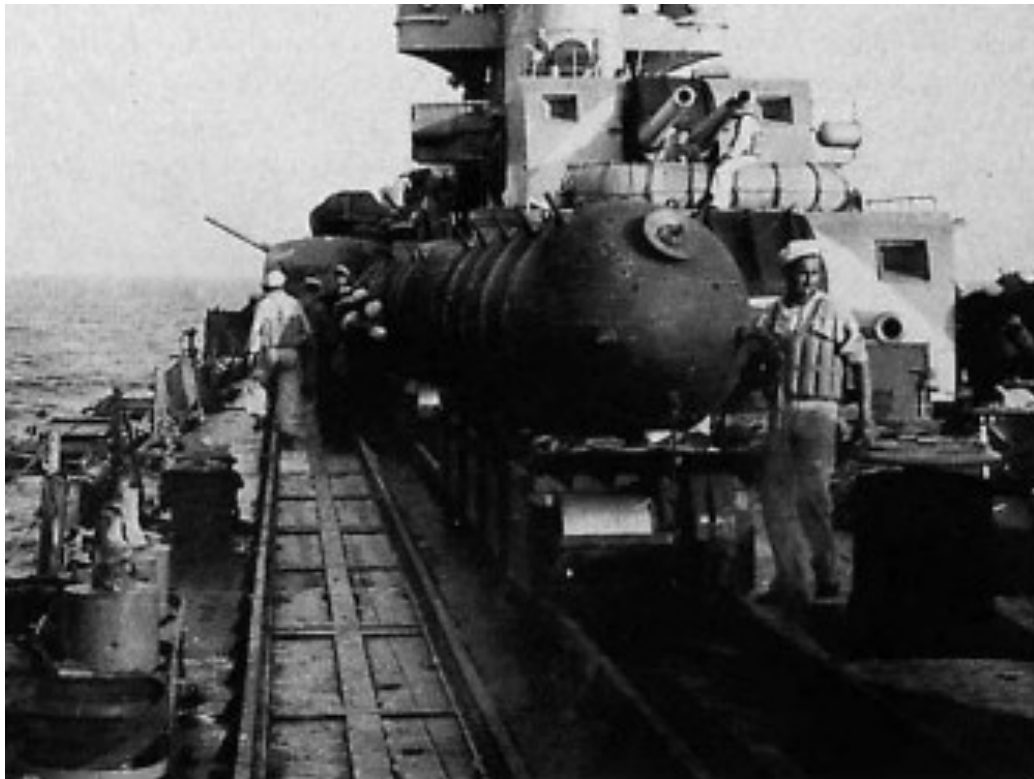
Mines and mine rails on an unknown early Condottieri class cruiser. The very close spacing of the M1926 OTO 152mm guns is clearly visible. Date unknown. (Courtesy USMM)
